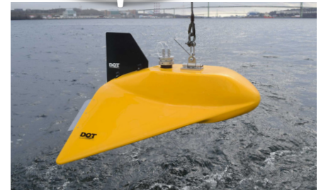
Phosphate Sensor and Reagent Housing deployed on a V-Wing. Powered from EM tow cable
