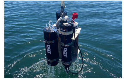
Autonomous deployment on a seafloor/river bed deployment frame
