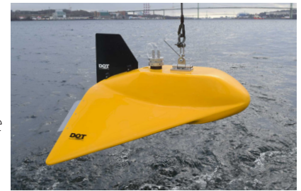
Sensor and Reagent Housing deployed on a V-Wing 1220, powered from EM tow cable
