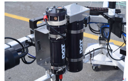
Nitrate & Phosphate Sensor and Reagent Housing mounted on Multi-Sensor Seafloor Platform (MSSP) by COVE
