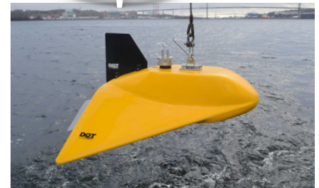
Phosphate Sensor and Reagent Housing deployed on a V-Wing. Powered from EM tow cable
