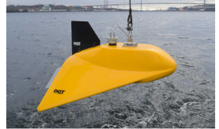
Sensor and Reagent Housing deployed on a V-Wing 1220, powered from EM tow cable
