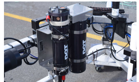
Nitrate & Phosphate Sensor and Reagent Housing mounted on Multi-Sensor Seafloor Platform (MSSP) by COVE
