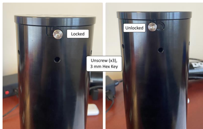
Figure 4: Reagent housing – lid removal
