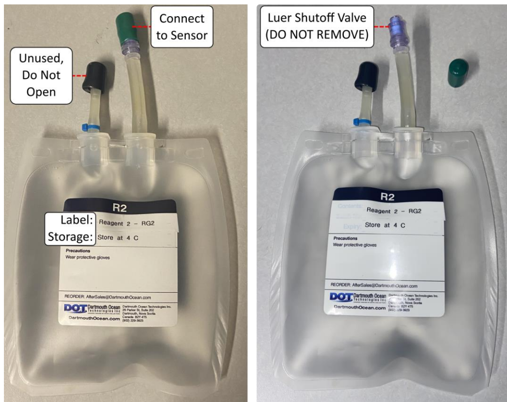
Figure 3: Fluid reservoirs. Connect green-capped tube to Sensor. NEVER remove purple valve.
