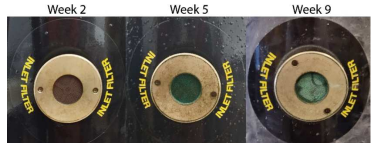
Fig. 1. Inlet filter of one autonomous eDNA sampler (Dartmouth Ocean Technologies, Canada) after being submerged in the Bedford Basin at weeks 2, 5, and 9 during the experiment. The centre of the inlet contains a copper mesh screen to filter out large particles and prevent biofouling. Over the duration of the experiment the inlet screening did not experience any biofouling, but did develop a patina that could potentially clog the inlet over long periods.
